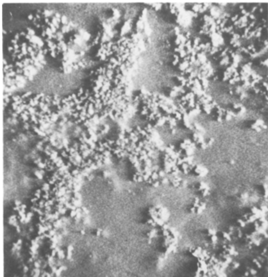
Figure 3 Scanning micrograph of a Au coated sample of glaze; \times 4000 , 30 kV.
