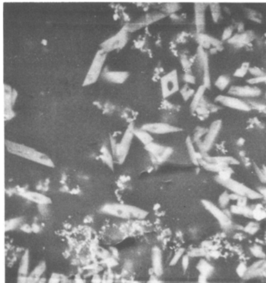
Figure 4 View of an area on the glaze surface showing a high incidence of needle-shaped crystalline material; \times 2000 , 30 kV.
